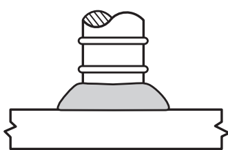
(C) COMPLETE JOINT PENETRATION GROOVE WELD—T-JOINT
